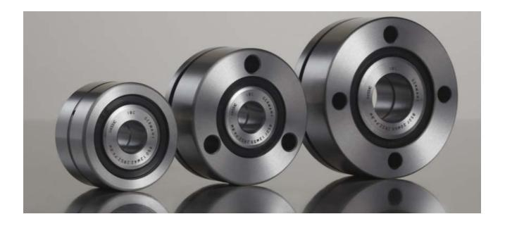
A double row 60° ball screw support bearing suitable for flange mounting (BSDF) is available, as is a type that is not suited for flange mounting (BSD). In the case of the BSDF ball screw support bearing, through holes in the outer ring enable you to flange mount the bearing directly to the adjacent construction or into a radial positioning boring. This will save time, because you will be able to dispense with the adjustment procedure.
